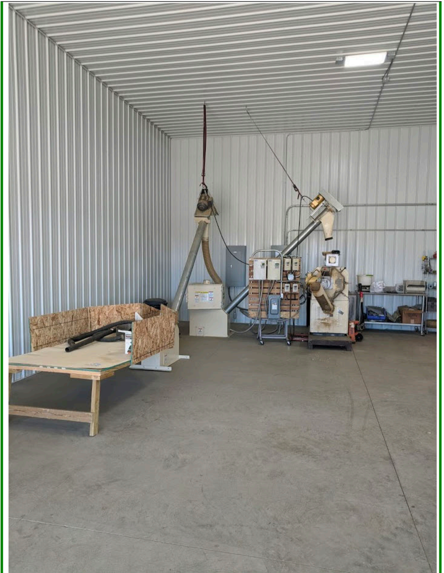
Pic 2: Accumulation table, hammer mill, and pellet mill. Vacuum sealer is behind the pellet mill.
