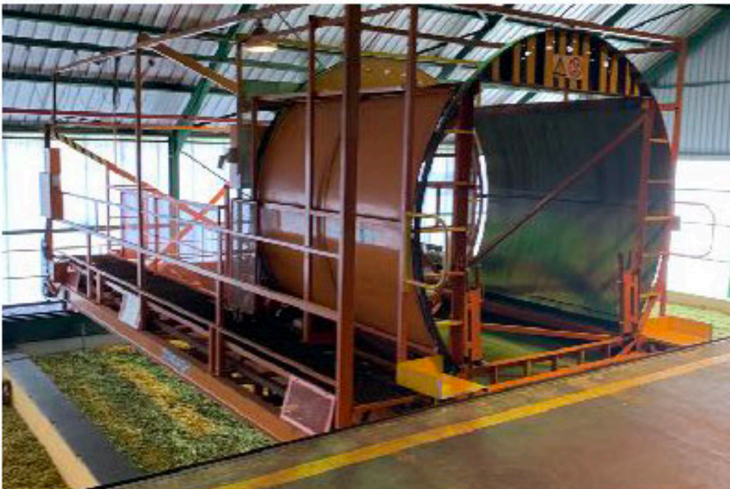
DRUM THAT DUMPS BINS OF HOPS INTO KILNS
